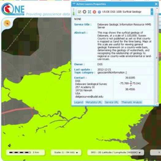
The resultant custom map (with the GeoSciML-Portrayal filter for Pleistocene polygons applied)
